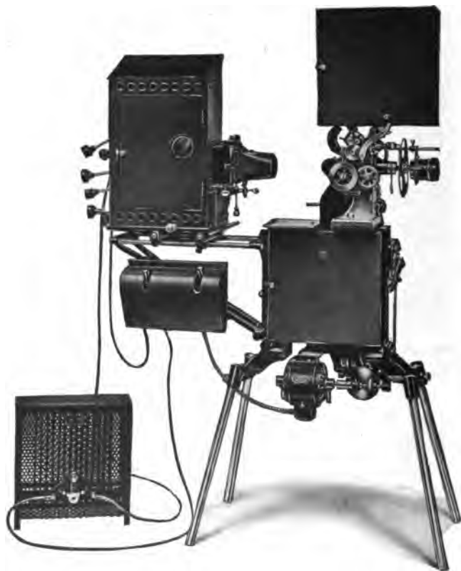
Powers Cameragraph No. 6A Showing rheostat and motor connections
